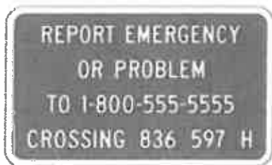
Figure 8B-5. Example of an Emergency Notification Sign
